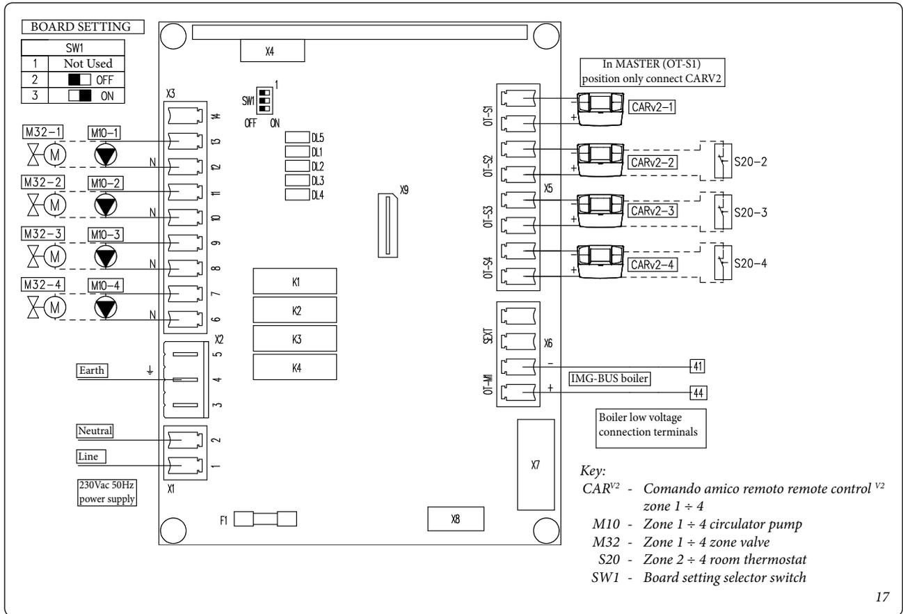
**Multi-zone kit wiring diagram, configuration of 1 high temperature zone - 1 low temperature zone.**
