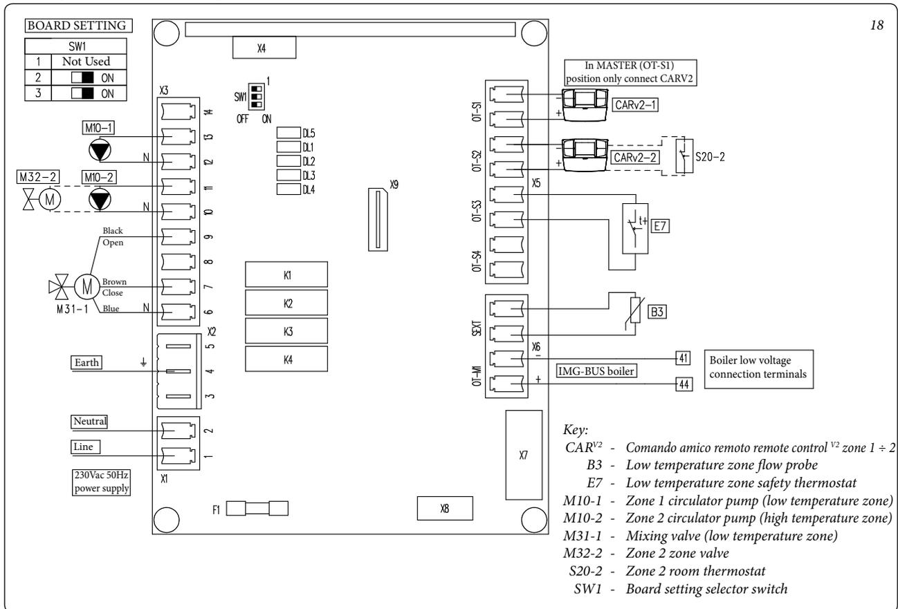
Wiring diagram of 2 multi-zone kits, configuration of 2 low temperature zones - 1 high temperature zone.
